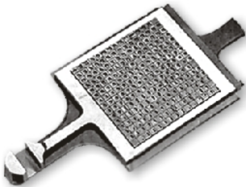
Fig 8.4 The Type Moulds Moulds for 225 different characters are contained in the frame
