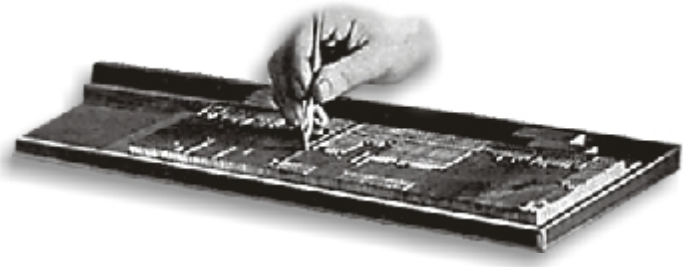
Fig 8.5 Gallery As the type is placed in its consecutive order it is passed into a long channel or 'gallery' where it is broken up into pages or any desired form. Corrections are also made at this stage.
